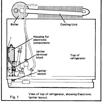
The size of the wire used to connect the battery to the igniter terminal block (fig.1), should be at least 0.75mm<sup>2</sup> in cross-sectional area. Correct polarity must be observed, - the '+' and '-' terminals of the battery must be connected to the similarly marked terminals of the terminal block.
